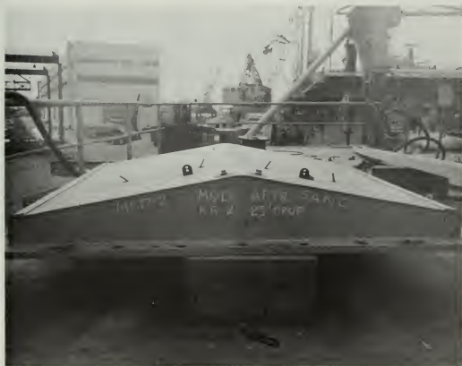
Figure L Model Backed by Sand and ML-D2 After 25 Foot Drop
